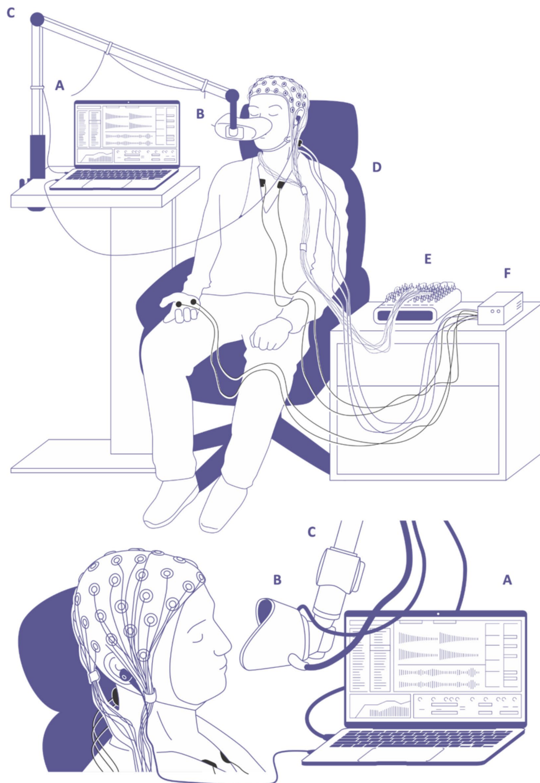
Fig. 2. Top Panel: Illustration of the experimental setup, showing the (A) MacBook running Ableton Live 10 and outputting audio through Sony XBA-100 earbuds and visual composition information to (B) ELA device affixed to the desk via a (C) M! ka arm mount swivel while participants sat in (D) a powered recliner. All participants were connected to a 64-channel EEG with a (E) dual-amplifier and a suite of bioperipherals connected to a (F) receiver. Bottom Panel: Profile view of the ELA device placed approximately five inches away from the participant's closed eyelids using the mount.
